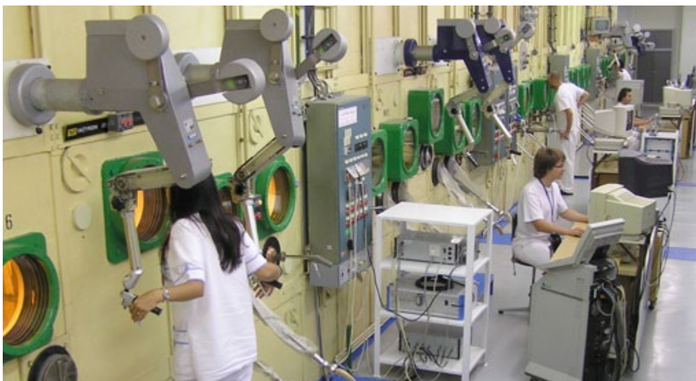
Current hot cells for material testing in NRI Rez (mother company of RCR)
